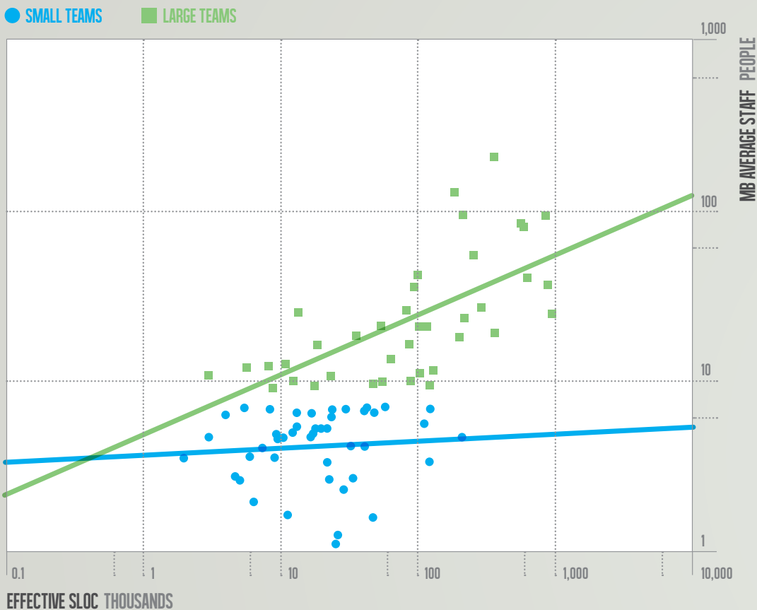
Figure 1: Plotting the number of lines of source code (SLOC) against the average staff sizes of "small staff" and "large staff" Agile projects.
